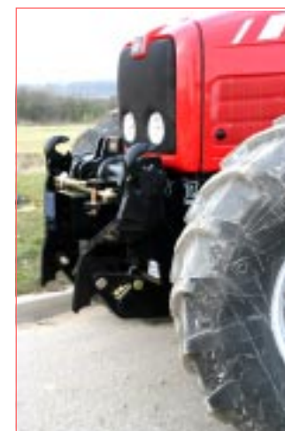
MDI 4 Folded. Minimal overhang from the front face.
